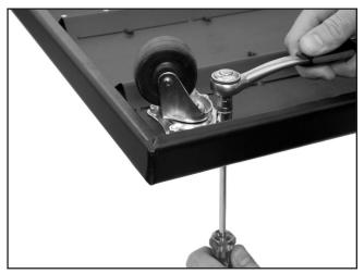
Figure 5. Installing casters.
